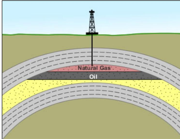
**Figure 1.1: Schematic of conventional oil and gas reservoir. Notice the accumulation of oil and gas in the high porosity sandstone layer (shown by the dotted layer) and the trapping of the oil and gas by the low porosity shale layer (shown by the dashed layers). The oil and gas is trapped in a geologic structure known as an anticline.**
