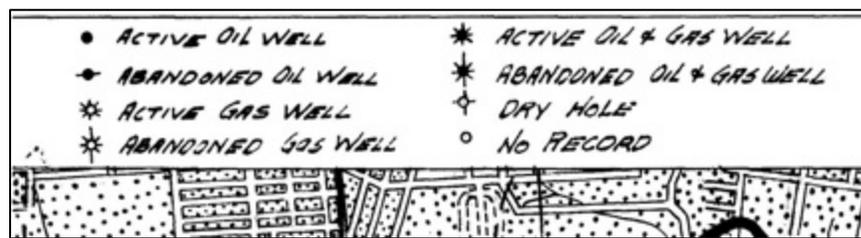
Figure 2.2: Legend of a WPA Bituminous Mining Map denoting the symbols for active and abandoned oil wells, active and abandoned gas wells, active and abandoned oil and gas wells, and dry holes.
